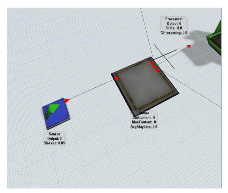
The above image shows how to view simple statistics for each object. If nothing is showing or only the names are showing, you can change the <u>View Settings</u> to show the statistics. To change the <u>View Settings</u>, click somewhere in the background of the view and in the Quick Properties window to the right, change the Show Names combo box to Show Names and Stats.
